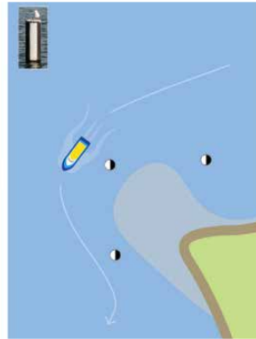
POINT BUOYS Identifies potential hazards between buoy and the closest shore.
